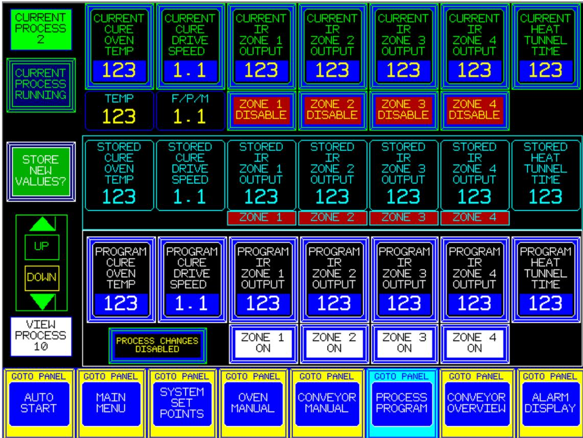
Each Process 1 through 4 may have a different Infrared Intensity programmed for it. These Process setpoints are then engaged from the Paint booths by depressing the black buttons or by entering a number from the **Booth Display** screen.
