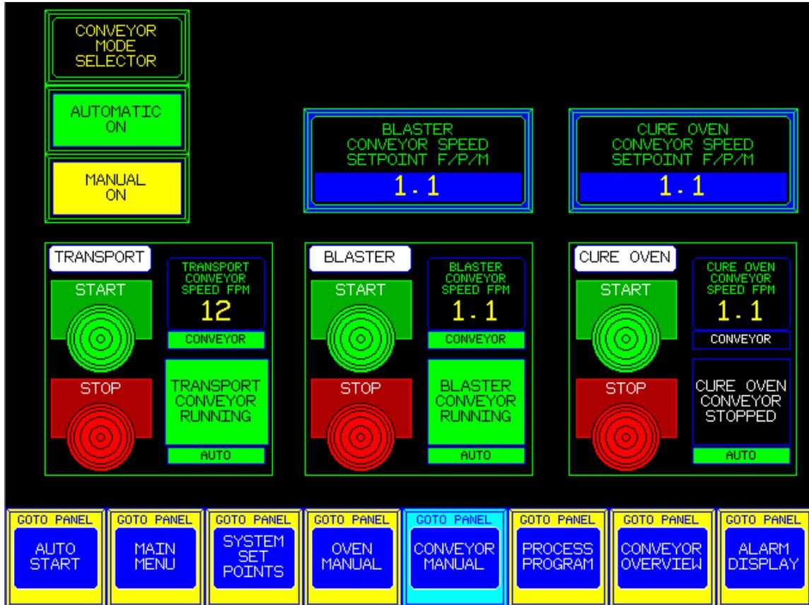
The Current Conveyor Speeds are displayed on the **Auto Start Screen** or the **Conveyor Manual Screen**.
