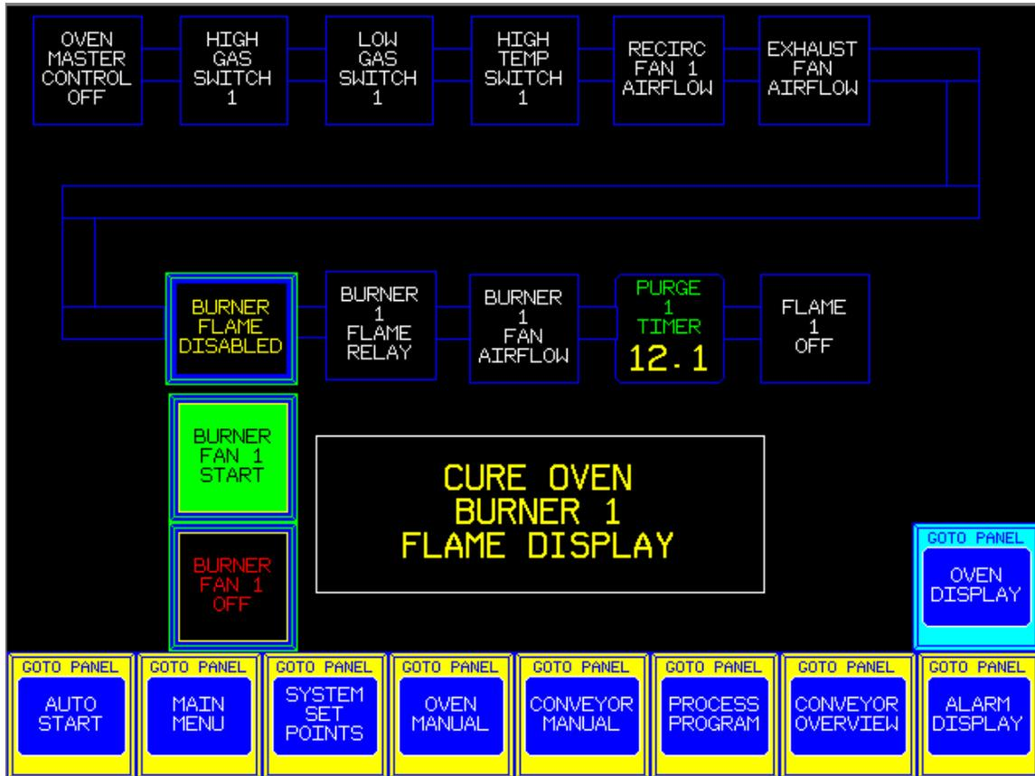
Each of the Flame Safeties are field wired in series, hence each must turn green on the Display Screen sequentially starting from the **Emergency Stop Input, Master Control**.
