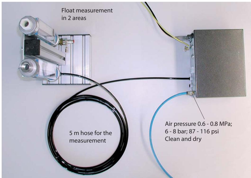
The comparison measurement should be within  $0.2 \text{ m}^3/\text{h}$  of the limit position. If the values are too far apart or once a valve has been replaced, the device can be recalibrated (see parameter C42, chapter 10.4).
