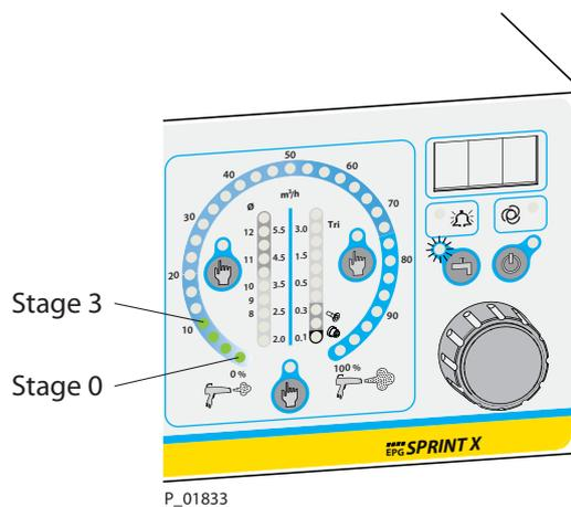
The "Powder Quantity" LED display 33 displays the offset stage currently used as point, e.g., the first LED lights up if stage 0 is selected.
